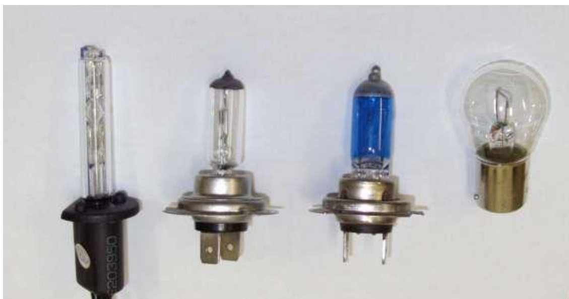
Figure 1. Different models of automotive lamps available in the market (from left to right): 35W Lamp HID xenon bulb, 55W halogen headlight bulb, 100W halogen headlight bulb, 21W conventional bulb.
