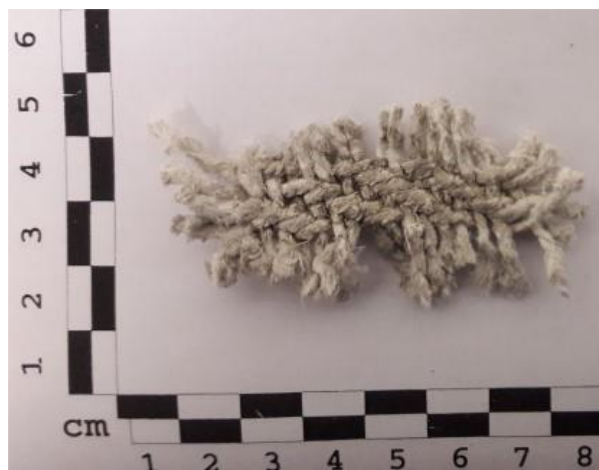
Figure 1. Part of the suspected sample that comprised the thermal insulation.
